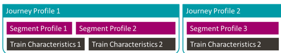
Figure 8: Illustration of AoE Data Packets
